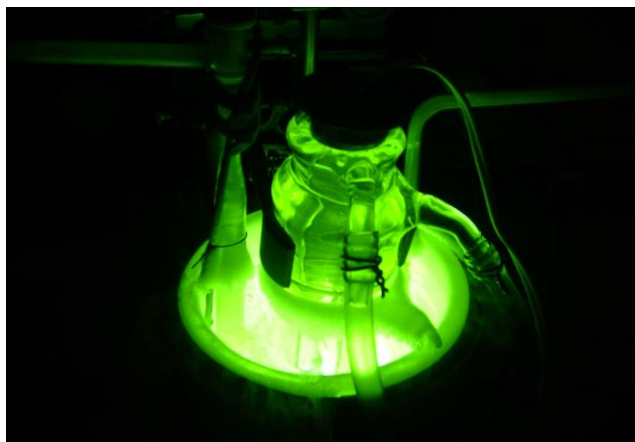
The photochemical synthesis of \text{KrF}_2 by the UV irradiation of a mixture of solid krypton and liquid fluorine carried out at liquid nitrogen temperatures [3,6].
